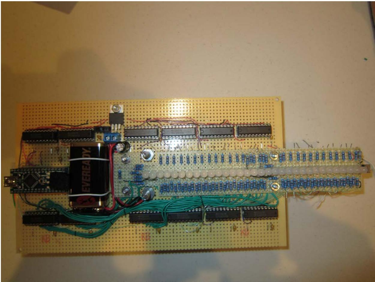
Main board with the LED board mounted on it.
