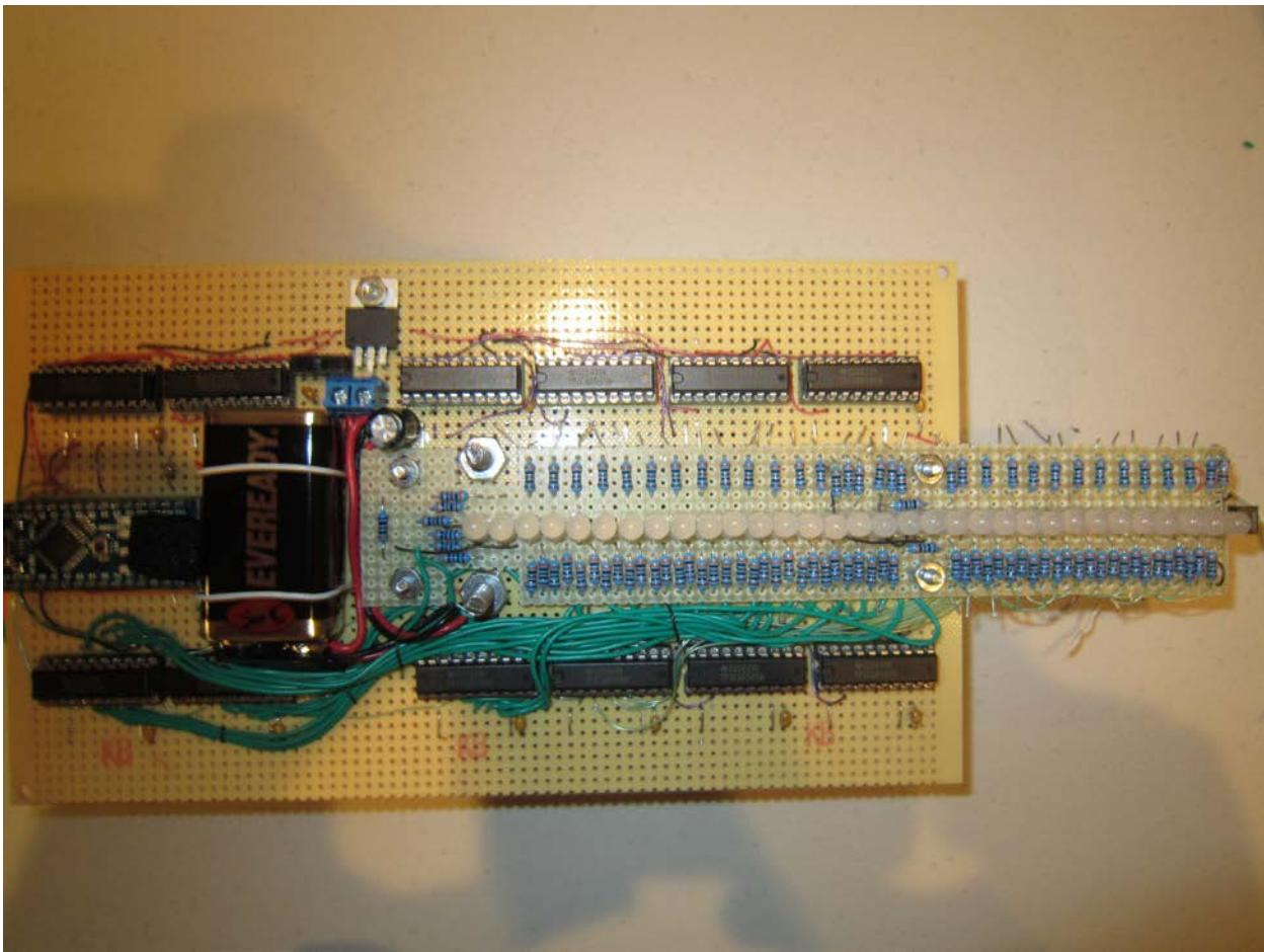
LED board showing the 32 RGB LEDs.
