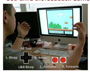
Advancer Technologies' last tutorial guided readers through the process to make a muscle sensor game controller that is able to play computer game by flexing their muscles. This controller uses the same sensor technology as the Bionic Armor but with a total of four sensors to give the user six-button gameplay control. Their YouTube demo video of the controller went viral and garnered over 140,000 views in a matter of days.
