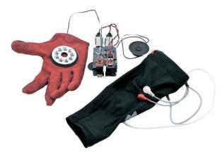
Advancer Technologies' "Bionic Iron Man Armor" harnesses the power of electromyography to give fans the power to directly control an Iron Man repulsor ray simply by flexing their muscle. When the wearer flexes their muscle, the Bionic system will play the harrowing repulsor charging-up sound effect from the Iron Man movies. Then, when the muscle is relaxed, the repulsor will emit a repulsor firing sound effect and flash on the LED lights attached to the palm of the glove.
